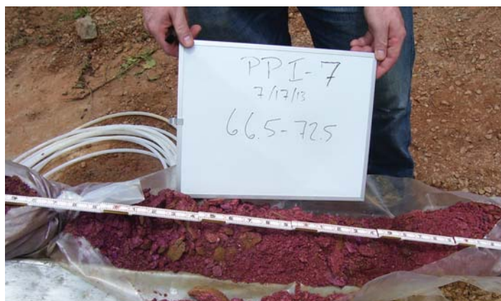
Figure 9. KMnO 4 persisting in saprolite at depth two years after injection
