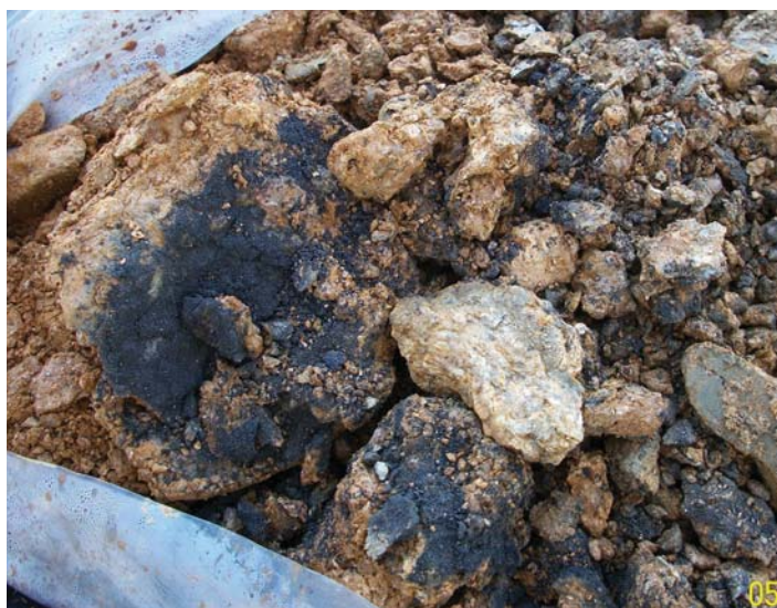
Figure 11. ZVI in soil cores from test boring
