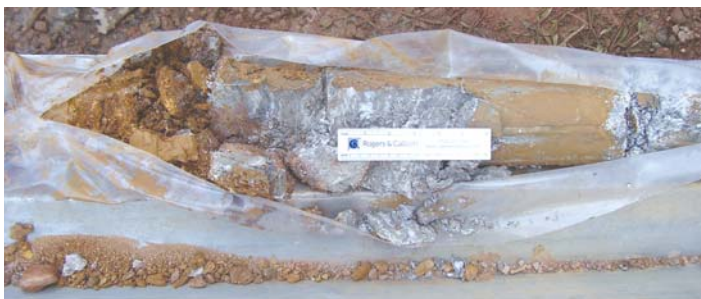
Figure 3. Low permeability saprolite
