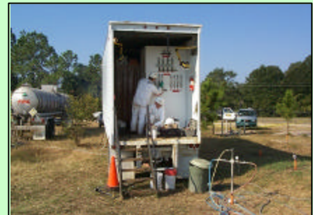
Figure 2: Process controls and catalyst in tractor-trailer and hydrogen peroxide in tanker truck.
