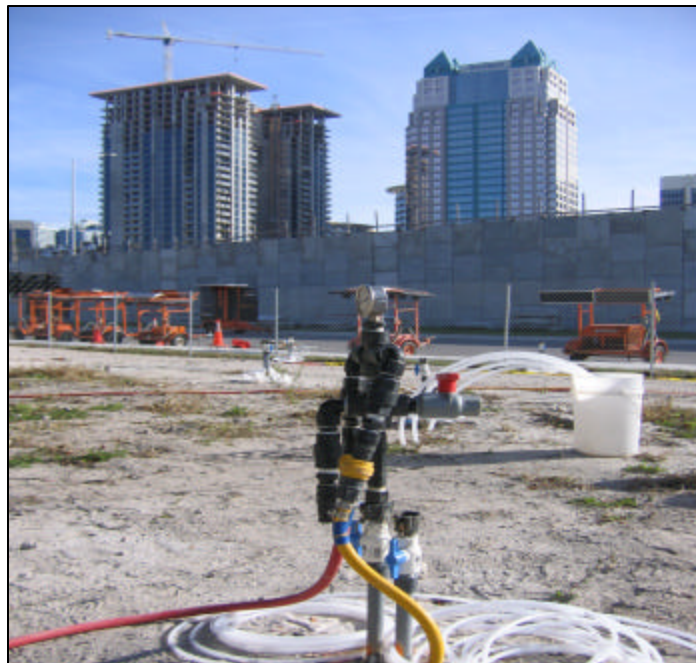
GCI'S PATENTED INJECTION DELIVERY STATION
